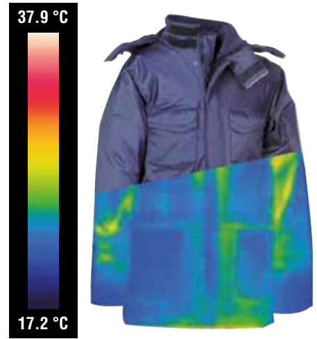
the light-blue colour proves the lack of escape ways for the hot air.
