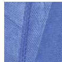
ultrasonic thermo-welded stitchings
